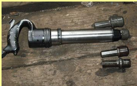
29/05/2010 - Newly acquired riveting tool, with a selection of heads.
