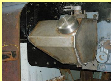
05/06/2010 - Newly manufactured sandbox awaiting finishing, temporarily bolted to frames.
