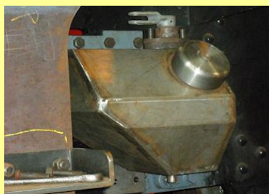
05/06/2010 - View of new rear right hand sandbox as bolted to the frames.
