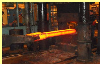
16/12/2010 - Ingot formed as a rear coupling rod.
