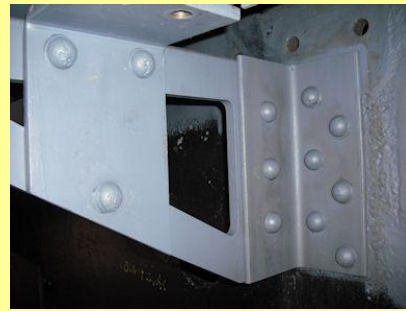
06/08/2010 - Front step riveted in place on buffer beam.
