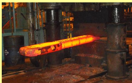
16/12/2010 - Coupling rod billet being lifted from furnace.
