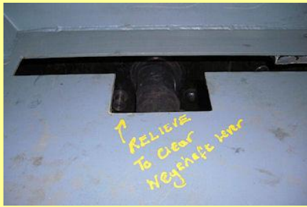
29/05/2010 - Slot cut into running plate to allow the wayshaft lever to be fitted.
