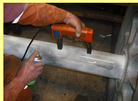
15/05/2010 - MPI testing the bogie wheel axles - passed successfully.
