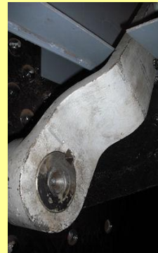
11/09/2010 - Modified link hanger bracket almost ready for fixing to frames.
