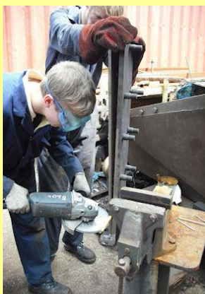
17/07/2010 - Cleaning the reverser pedestal after stripping from remains of the much rusted and useless reverser tower.
