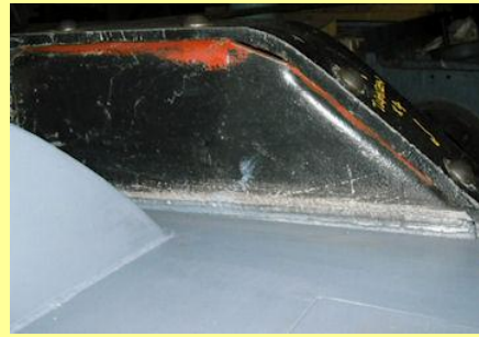
29/05/2010 - Correct round headed bolts fitted to motion plate covers. The right hand motion plate cover has been modified to sit correctly on the frame valance.
