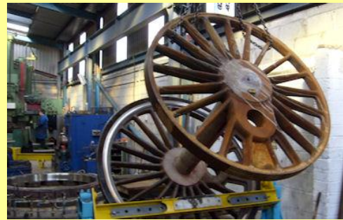
10/02/2010 - One tyre having been fitted, the wheel set is turned over for the other driving wheel to be tyred - the tyre being seen in the background. Clearly shown too, is the hole for the crankpin. (David Hurd)
