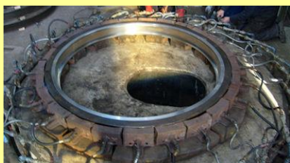
10/02/2010 - Machined tyre in gas ring furnace, being heated causing it to expand ( David Hurd ).
