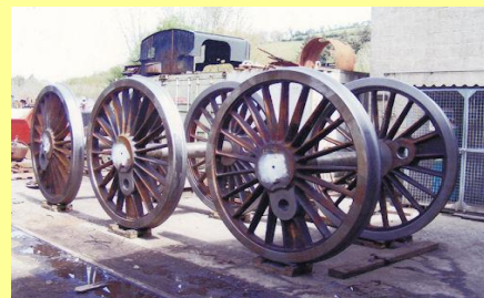
30/04/2010 - 1014's wheel sets at Buckfastleigh - essentially complete apart from fitting the crankpins. They will be transported to Didcot Railway Centre in the very near future. Wheeling the chassis is scheduled for June/July ( Jeffery Harper )
