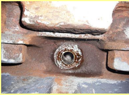
13/02/2010 - The valve chest drain - and the corrosion.
