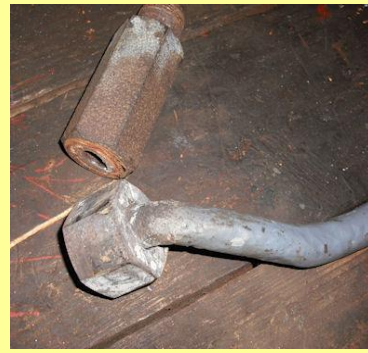
13/02/2010 - The one drain pipe that could be removed - corroded thread to be seen at the top edge of the image.
