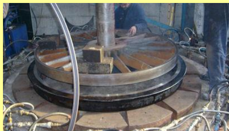
10/02/2010 -Wheel set being lowered into the expanded tyre. ( David Hurd )
