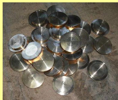
31/01/2010 - Completed sand core plugs.
