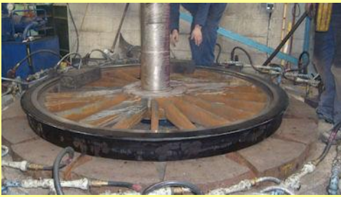
10/02/2010 - Wheel inserted into tyre - the tyre was then allowed to cool, thus contracting and firmly 'gripping' the wheel, to the point where it is immovable. (David Hurd)
