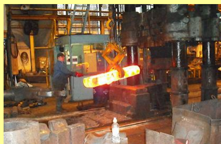
16/12/2010 - Ingot being carried to press.
