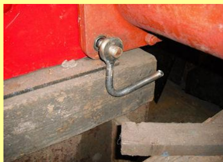
19/06/2010 - Newly manufactured coupling suspension hook placed on bolt holder of buffer.
