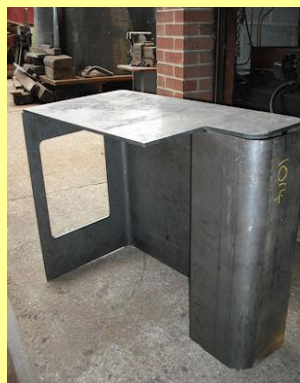
06/08/2010 - Steel to fabricate a new reverser tower after delivery and awaiting welding.
