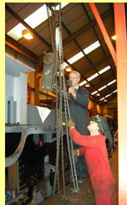
23/10/2010 - Lifting the reverser screw and pedestal onto the reverser tower.
