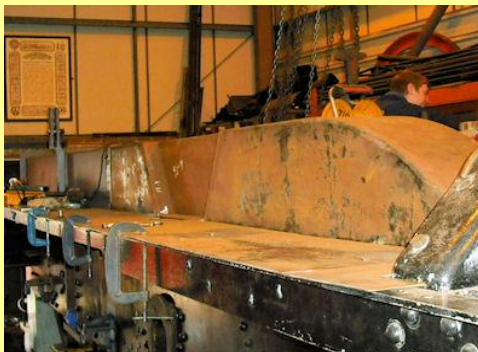
13/03/2010 - Right hand splashers aligned and ready for welding together and to the running plate.
