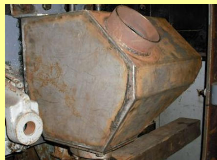
13/03/2010 - Newly fabricated left hand rear sandbox trial fitted to frames.
