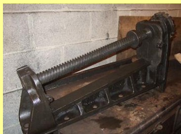
16/01/2010 - Removing years of gunge/dirt from the screw reverser.
