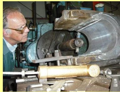
31/07/2010 - Machining a bogie bearing.
