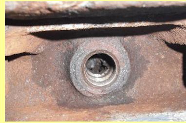
06/11/2010 - Nipple drain hole on the cylinder casting following removal of rusted remains of nipple. The thread has now been cleaned in readiness for inserting the replacement nipple and drain.
