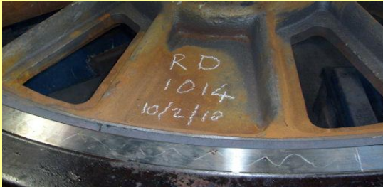
10/02/2010 - The evidence! 1014's driving wheel with tyre fitted. (David Hurd)
