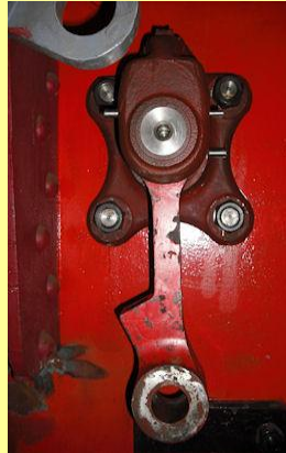
06/11/2010 - First link hanger bracket bolted (temporarily) to the frames. To complete the task spring washers are required, which are being acquired.
