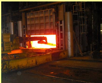
16/12/2010 - Coupling rod billet being lifted from furnace.
