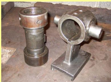
16/01/2010 - Reverser worm and bearing following cleaning.
