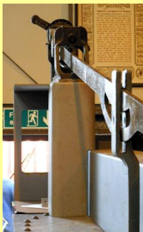
06/11/2010 - Reverser assemblage on footplate.
