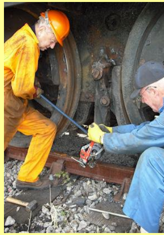
1-2/07/2010 - Chris C and Gary D. working hard to release brake hanger.
