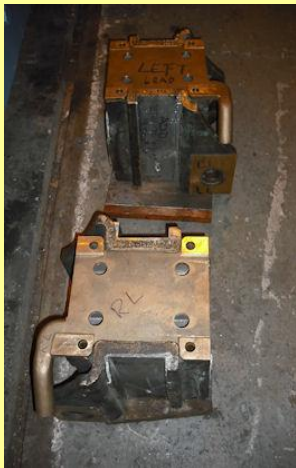
06/11/2010 - Oil keeps trial fitted to axle box bearings.
