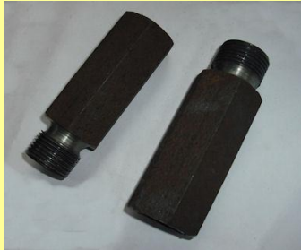
02/10/2010 - Newly manufactured cylinder drain nipples.
