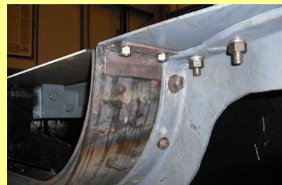
25/09/2010 - right hand side under-cab footplating fitted and bolted to running plate and valance.
