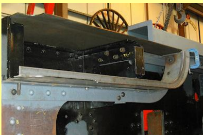
11/09/2010 - right hand side under-cab footplating being fitted.
