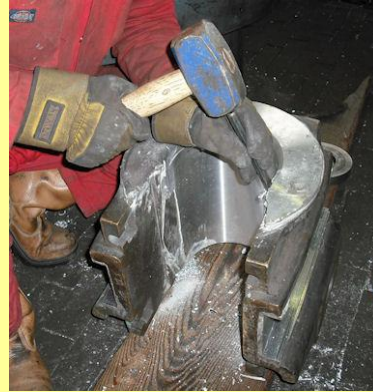
13/02/2010 - Fettling a machined bogie axlebox.
