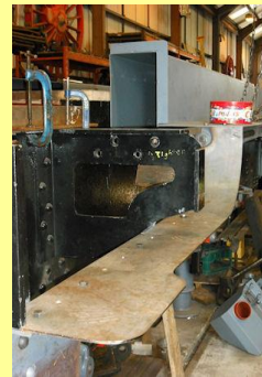
21/08/2010 - fitting the under-cab footplating in place - note too the primed sandbox.
