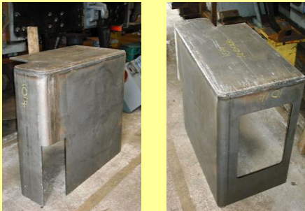
21/08/2010 - two views of the reverser tower following welding of the steel components.
