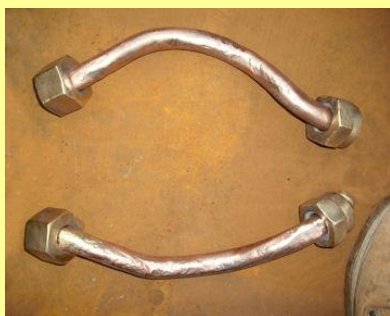
19/06/2010 - Cleaned steam chest drain pipes - scale can be ascertained from shoe at bottom right hand corner of image!
