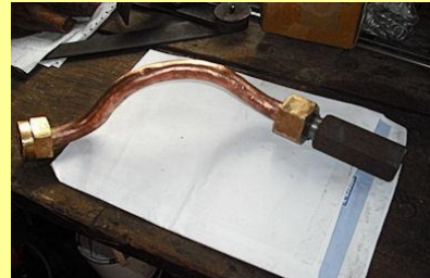
02/10/2010 - Refurbished piston valve drain pipe with new nipple attached.
