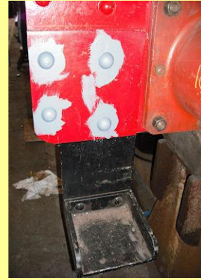
06/08/2010 - Front step riveted in place on buffer beam.
