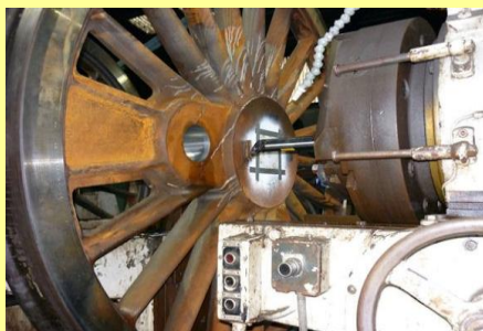
08/04/2010 - Drilling holes for the crankpins ( Dave Hurd )
