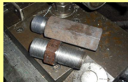
06/11/2010 - Newly manufactured larger nipples for fixing the drain pipe to the smaller nipples fixed into the piston valve chest.
