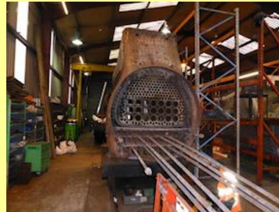
03/2017 - front end of the repaired firebox awaiting being joined to the boiler. (David Bradshaw)
