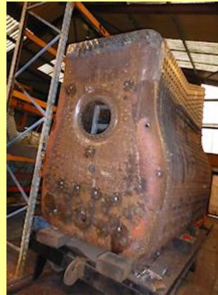
03/2017 - view of the cab end of the firebox showing renewal work undertaken.
