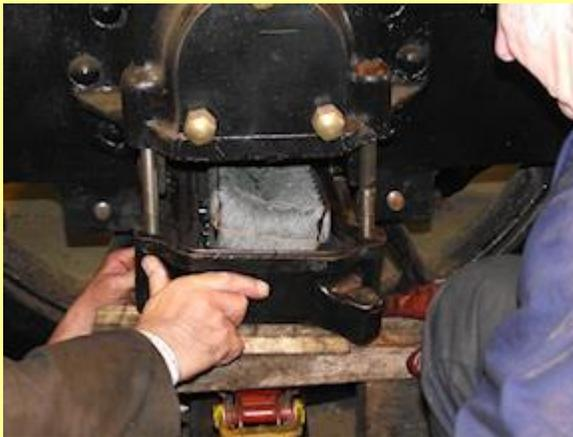
06/09/2017 - fitting lubrication pads to tender axleboxes.
